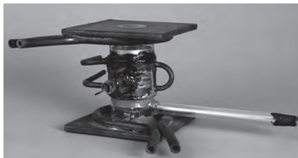
Fig. 6 – First Magnetron prototype developed at Birmingham in 1940.
